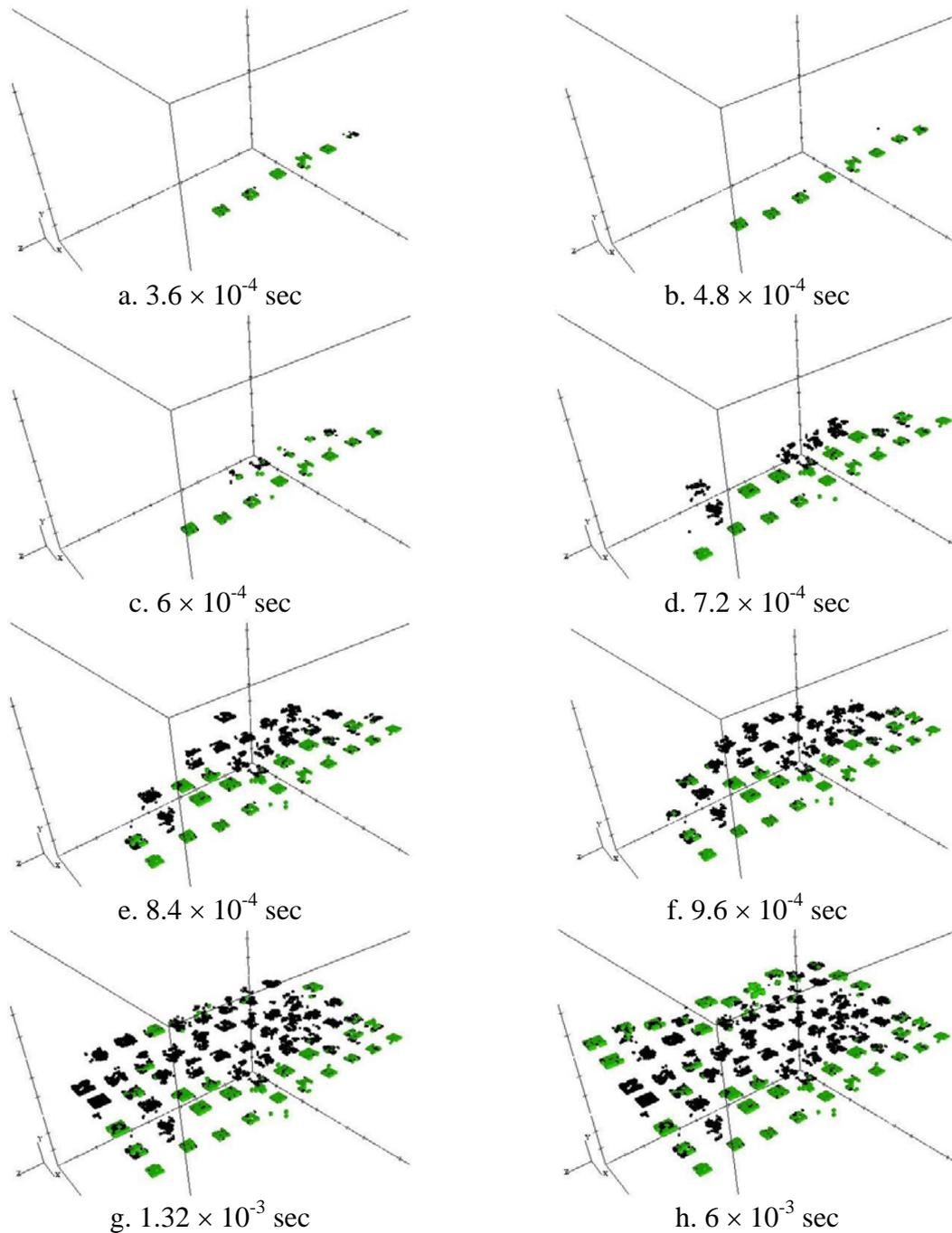
FIGURE 4. Fracture propagation on the CA scale at  $-30^{\circ}\text{C}$ . Only dead brittle (black) and dead ductile (green) cells are shown.
