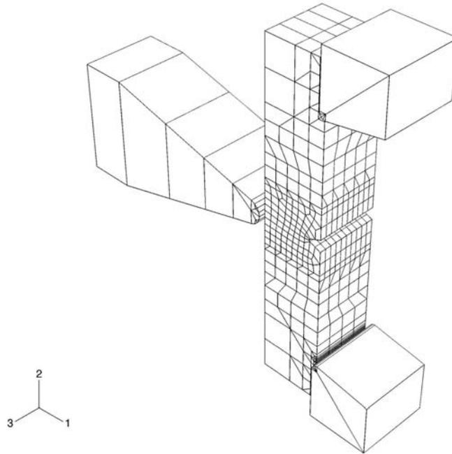
FIGURE 2. The finite element mesh of the Charpy specimen, the anvils and the striker.
