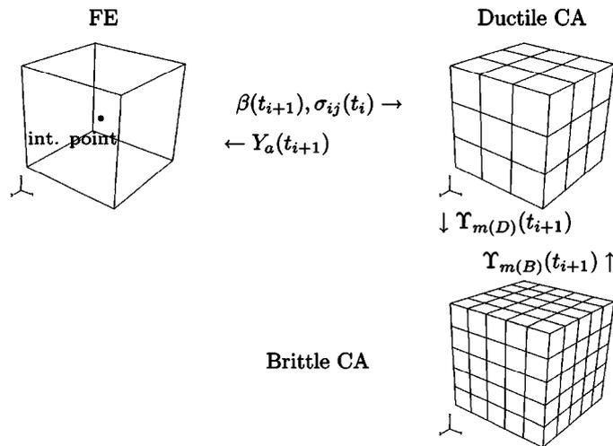
FIGURE 1. Flow of information between the finite element integration point and the ductile and the brittle CA arrays.
