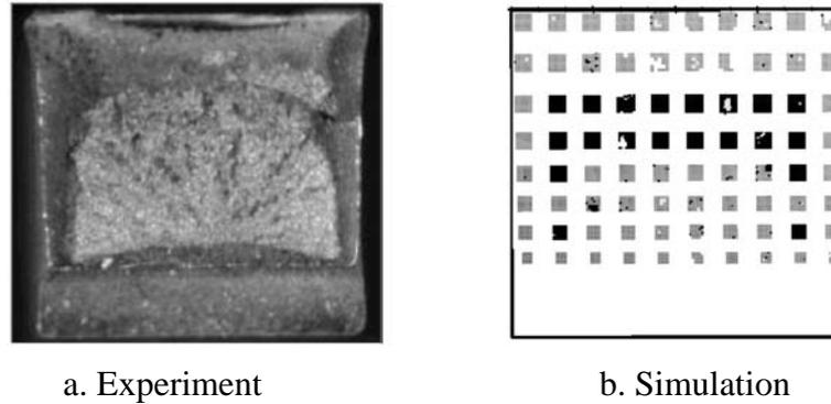
FIGURE 5. Experimental (a) and simulated (b) Charpy fracture surfaces. In (b) the black colour denotes brittle fracture and grey, the ductile fracture.
